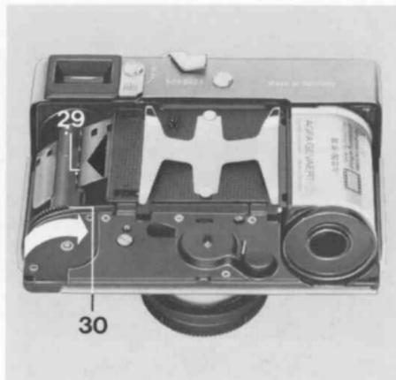
Push the film leader fully through the slot **29** and wind it up on the take-up spool by turning the milled wheel **30** in the direction of the arrow until it stops.
